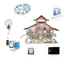
In addition, the company is constantly involved in developing new innovative solutions for new line of products. As an example, Oblo Ecosystem is a set of hardware and software components which enables remote light control, as well as power consumption monitoring in a Smart Home concept, through the TV, PC, mobile phone, from home or any other place with access to the Internet (http://www.rt-rk.com/new/oblo).
