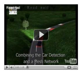
Roadnail product offers road marking based on sensors, wireless connectivity, energy harvesting and light marker as well as local intelligence. It is used to make visible the edge of the road in the front view of a moving car. The system does not need any equipment in the car and therefore works with current car fleet. It is powered autonomously by solar cell on the top of each devices (<a href="http://www.rt-rk.com/new/roadnail">http://www.rt-rk.com/new/roadnail</a>).
