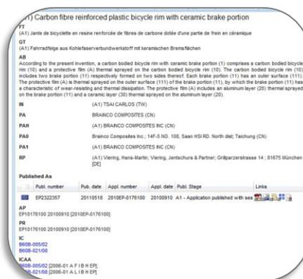
**(A1) Carbon fibre reinforced plastic bicycle rim with ceramic brake portion**
