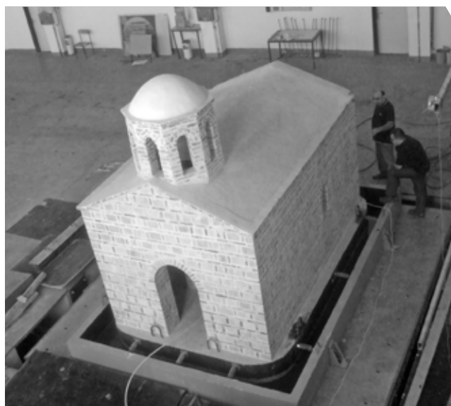
▲ Shaking table test at the Institute for Earthquake Engineering and Engineering Seismology, Skopje, (picture provided by: Assoc. prof. dr. Lidija Krstevska)
