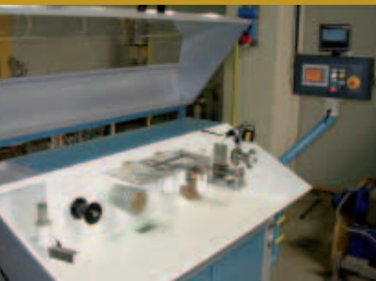
A laboratory drawing machine for ultrathin wires developed by CNR-IENI (Italy).
