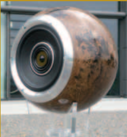
Loudspeaker box made from a lignin matrix composite.
