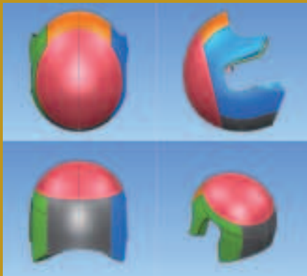
Safer customised motor cycle helmet with an inner lining that has been designed to fit the scanned shape of the rider's skull.
